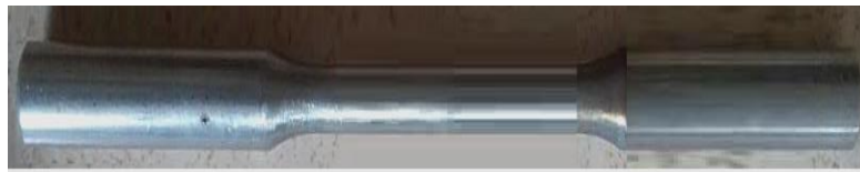
Figure 2. Tensile Test Raw Without Welding Specimen
